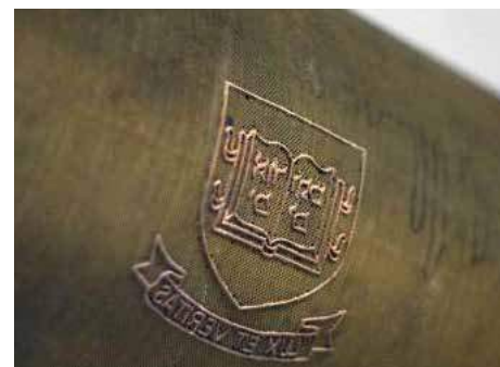
Example of a dandy roll for single-tone watermark on Fourdrinier machine.
